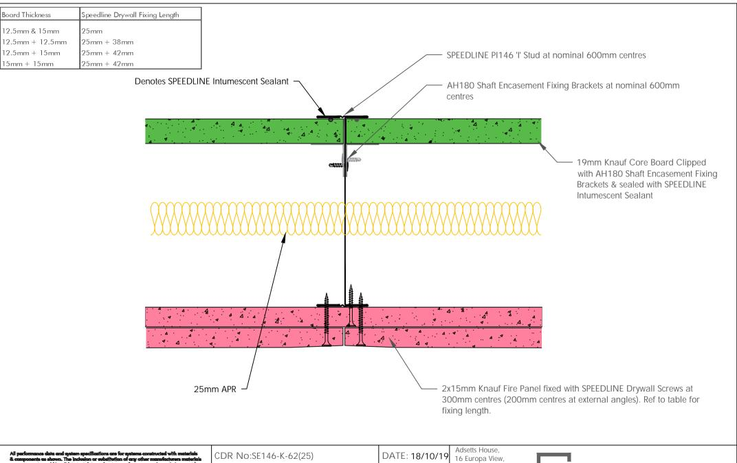
SHAFT ENCASEMENT PARTITION SYSTEM TWO BOARD LAYERS - 146mm STUDS
